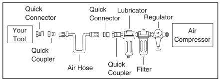
Figure 2. Typical filter/lubricator/regulator installation order.
